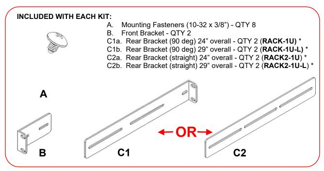
\* NOTE: Only one set of rear brackets is included per kit. Select either RACK-1U, RACK-1U-L, RACK2-1U, or RACK2-1U-L.
