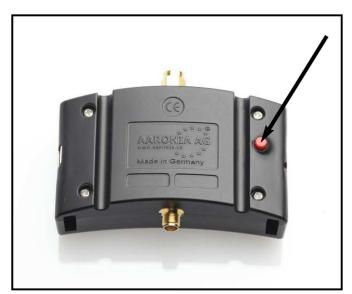
The UBBV-preamplifier can be turned on and off at the switch on the back side of the preamplifier. With the integrated LiPo-battery the preamplifier has a runtime of approx. 3-4 hours.
