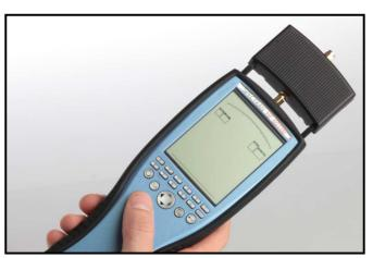
**ATTENTION:** If you don't use the SPEC-TRAN together with our LCS or MCS software, you have to activate the UBBV-preamplifier in the menu "RefOff" (by choosing the headword "UBBV12") in order that the SPECTRAN is calibrated correctly!
