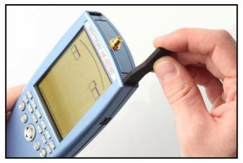
Please put the enclosed mounting brackets consistently and in a non-violent way in the intended slots of the SPECTRAN until it locks firmly.
