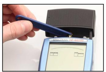
Please leave always, if possible, the both devices connected as every removal and re-assembly could wear out the SMA jacks and could cause damages!
